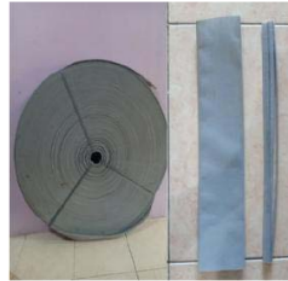
Figure 2. Prefabricated Vertical Drain (PVD),
