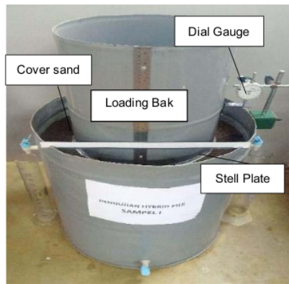
Figure 7. Test equipment installation position
