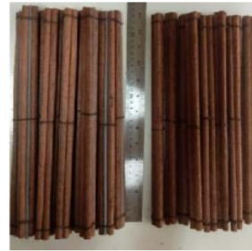
Figure 3. Timber Pile and Timber pile+PVD (hybrid pile)
